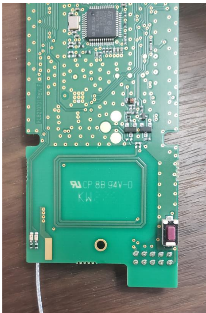
Transistor interface for the near field loop. Bottom right is the power button. Bottom left are status LED's. Wire at the bottom left is the 400MHz antenna.
