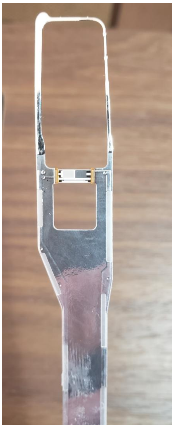
Close up of temperature and humidity sensors. The loop is a platinum RTD temperature sensor
